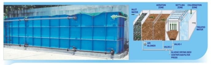
The INDION Fluidised Media Reactor (FMR) is designed as a single tank unit, incorporating a bar screen chamber, specially developed synthetic media to facilitate attached growth process, oxygen transfer through diffused membrane aeration, a lamella settler and a chlorine contact tank for disinfection.
